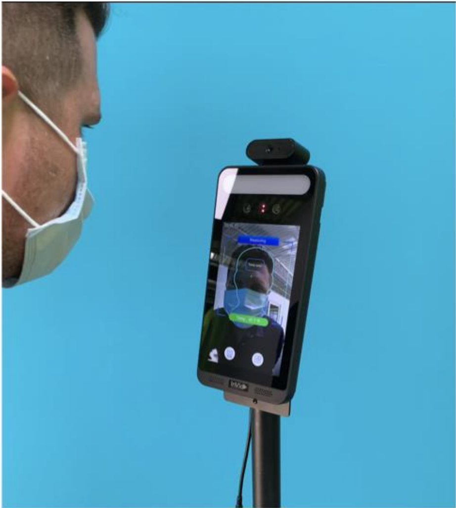
Can be programed to provide mask compliance so the door doesn't open without the employee putting a mask on. Can be used to avoid violations/citations.
